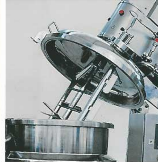
K Mix platform 300 litres CIP/SIP gear box with 2/3 bar mixing 2 bar high flow / low shear homogeniser Manual vacuum / pressure / N2 Pneumatic bottom valves Direct heating/cooling, CIP/SIP system
