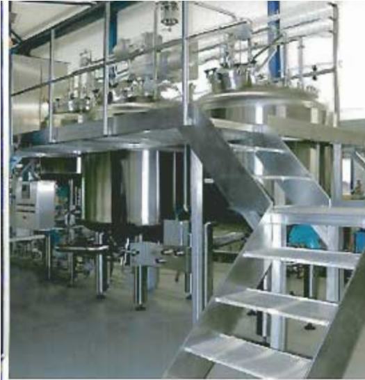
MMS Platform 2500 litres CIP/SIP gear box with 2/3 bar mixing 2/3 bar high flow / low shear homogeniser Automatic vacuum / pressure / N2 Integration of different phase vessels Indirect heating/cooling, CIP/SIP rack
