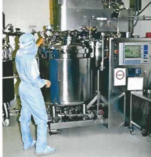
MMD Platform 500 litres CIP/SIP gear box with 2/3 bar high speed mixing Automatic vacuum / pressure / N2 Cooling mechanical seals GAMP 4 software Direct heating/cooling, CIP/SIP rack
