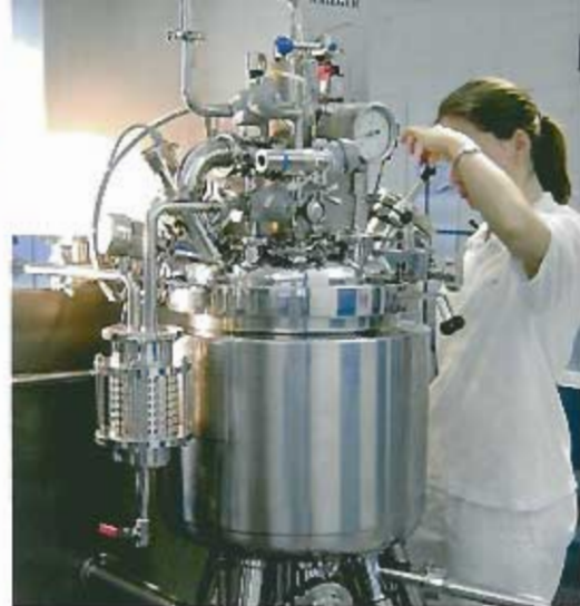
MMD Platform 30 litres CIP/SIP gear box with 2/3 bar mixing 2/3 bar high flow / high shear homogeniser Automatic vacuum / pressure / N2 Alex design Indirect heating/cooling, CIP/SIP rack
