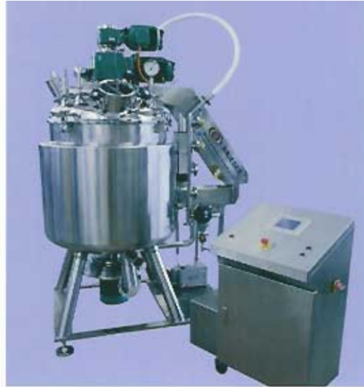
KMix platform 300 litres vacuum mixing process (-1/0.5 bar) 2 bar high flow / low shear homogeniser Manual vacuum / pressure / N2 Touch screen panel Direct heating/cooling, CIP system
