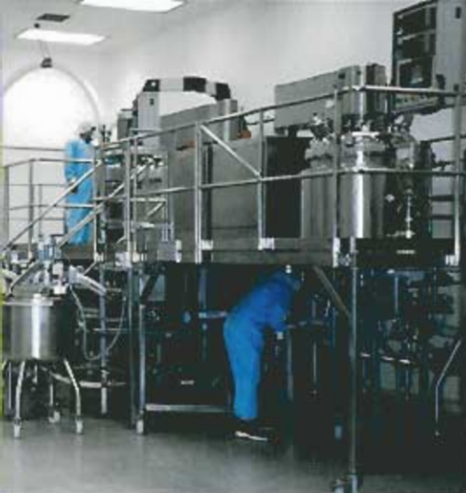
MMD Platform 700 litres CIP/SIP gear box with 2/3 bar mixing 2/3 bar high flow / low shear homogeniser Automatic vacuum / pressure / N2 Integration of different phase vessels Indirect heating/cooling, CIP/SIP rack
