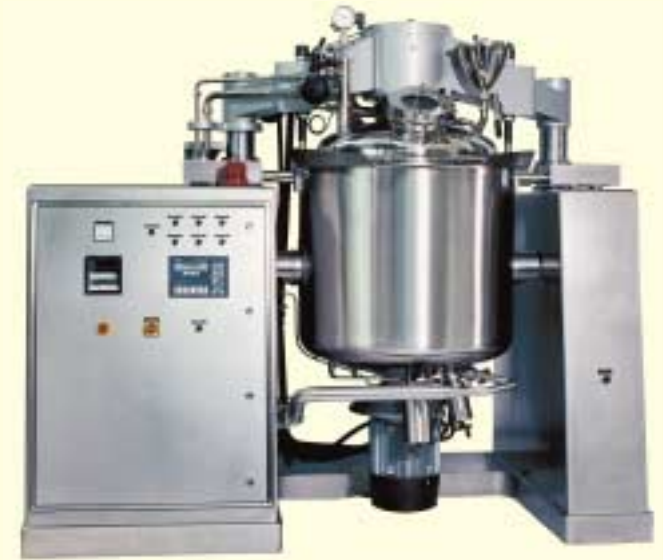
MMU with integrated CIP system. The CIP pump, recirculation pipework and water connections are integrated in the machine frame and comply with GMP requirements.
