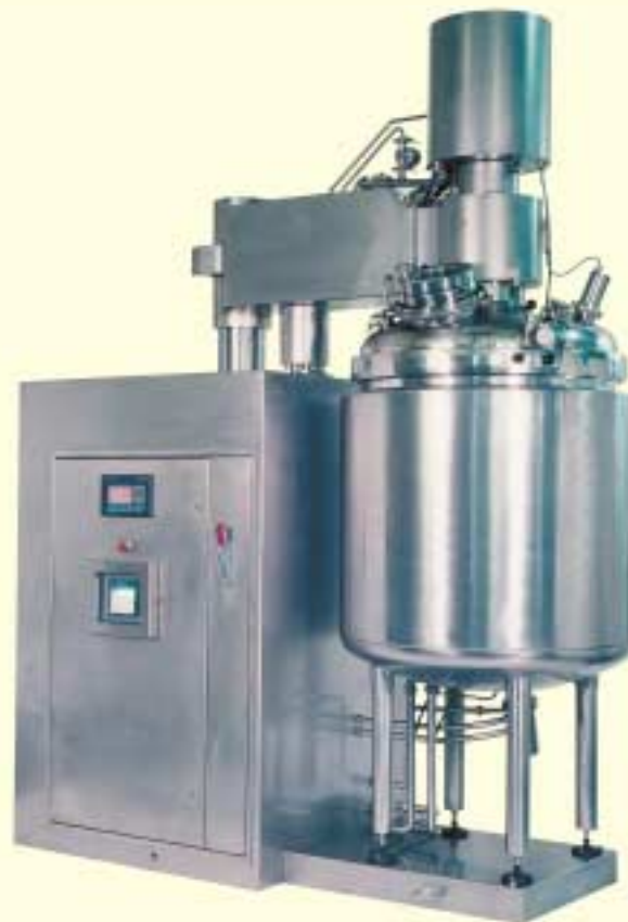
MMD 600 with outer agitating arm, high-speed shear blade and gearbox with controlled single sealing point. Fully sterilisable, used for ophthalmic applications.
