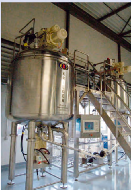
K- mix 2500 liters with automatic CIP System
